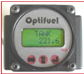
Above: Optifuel flow sensor. Below: The Optifuel indicator.
