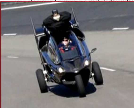
Below: The PAL-V flying surfaces folded on the road at speed showing the leaning feature of an already flying prototype.
