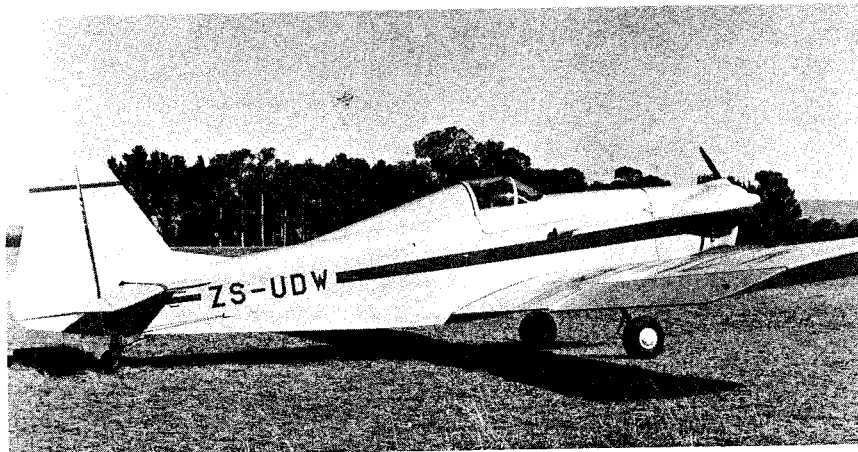
South African "Mini-Ace" built by H. C. van Rensburg. CA-61 has a 1600 VW engine which required lengthening the nose to compensate for the reduced weight when the VW was substituted for a Continental 65. The aircraft is beautifully finished in yellow with red trim.
