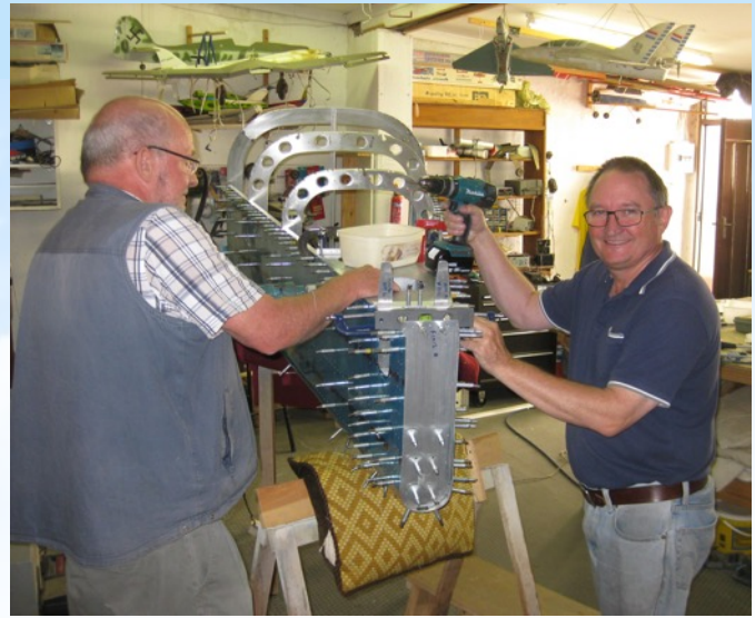
Clecos holding the tail cone together
