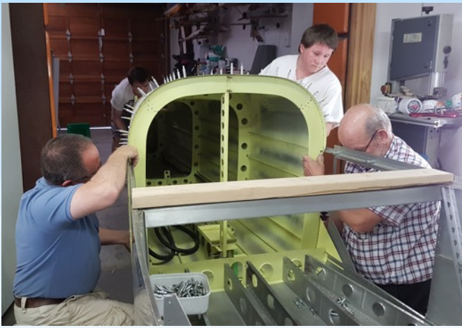
Joining the tail cone to the forward Fuselage- a big moment
